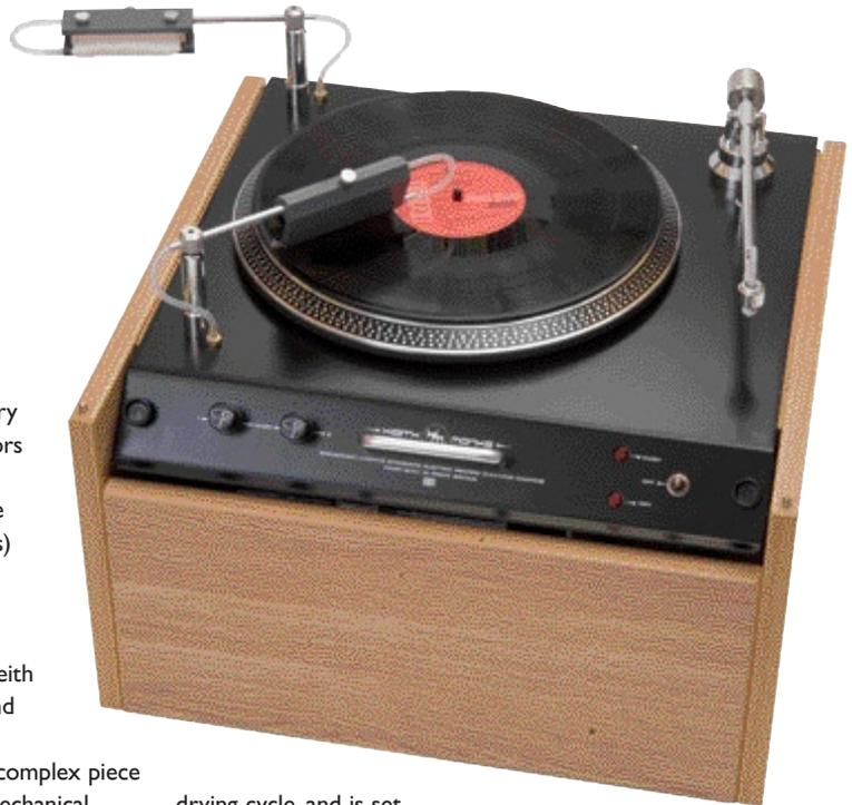
drying cycle, and is set to work at 20in Hg – in accordance with the original Percy Wilson design. Jonathon Monks adds that any more suction can exert too much force on the record and make the nozzle leave spiral marks on the disc. As with the arm drive motor, the suction pump only works on the dry cycle.
